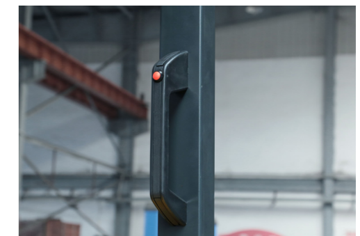
Back-up handle with horn button: improving both driver's comfort and reversing safety
