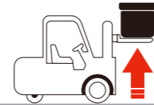
0.24m/s Max. lifting speed with load
