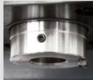
Stable piston rod (Ø 55 mm) with tool anti-twist device
