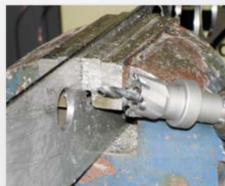
Free-hand drilling up to Ø 30 mm
