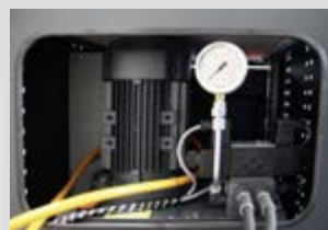
Dual-circuit hydraulic unit in cabinet base
