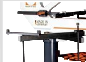
Pivoting support arms, height adjustable, each with 2 rubber supports
