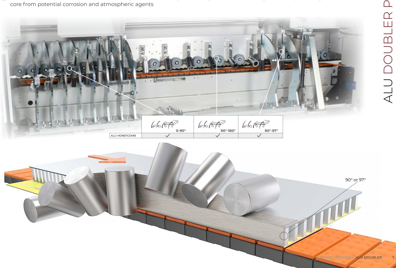
• The full process made by Alu Doubler F and Alu Doubler P with the manual punch press allows to otbain alu honeycomb panels with protected edges and corners
