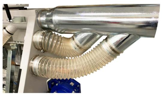
• Centralized hood suction system in a unique tube (Opt. LOAB31) allows to eliminate the wood chips through the suction system
