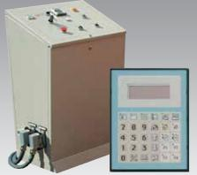
• The operator is able to control all machine operations using the control panel. The Multiprogram version allows to manage a list of up to 20 positions, with different quantities and lengths of rebar.
