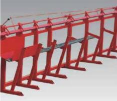
• Guiding support with a mechanical end-stop, for the manual regulation of cutting length. The bars cut to size are collected into a rack.
