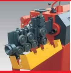
• The Multiprogram version has a pre-straightener unit consisting of five rollers and a pair of measuring rollers connected to an encoder. Cutting to length is electronically programmed, working according to pre-loaded cutting sequences. (OPTIONAL)
