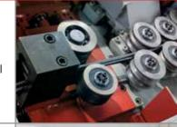
Motorized pre-feeding roller, for the insertion of the wires.
