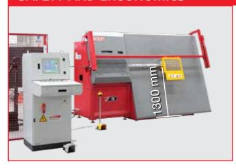
With the AFS2 system it is always granted to obtain closed stirrups, thus eliminating the typical and dangerous manual operation during the bending process by operator. It is possible to produce straight bars or bent at one end, in total security.
