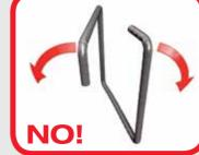
The twisting of the wire during the pulling phase creates open stirrups.
