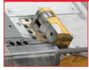
The cutting unit uses a universal knife, suitable for any type of diameter and provided with 4 cutting profiles.
