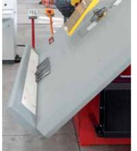
"TFS" allows to obtain always closed stirrup, eliminating the dangerous manual intervention of the operator during the bending phase. The exclusive design of the worktop, equipped with a lower collapsible element, makes it possible to produce large stirrups (maximum distance between the central pin and the flooris 1900mm ) as well as becoming a collection shelf for all the stirrups, thus avoiding their fall to the floor.
