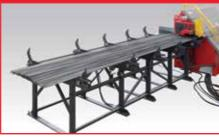
**F13 BAR** can be equipped with a stock rack with double automatic chains depending on the selected configuration. It allows the management of two bundles characterized by different diameters  $\emptyset 10 \div \emptyset 13$ , or of the same diameter  $\emptyset$ 10 but of different lengths 9 m - 12 m, in order to maximize the optimization by reducing the scrap.
