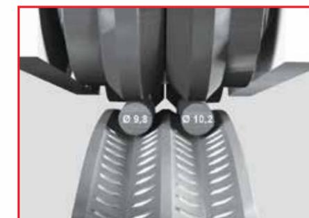
**The coil ribs deformity are reduced at the least without modify the mechanical characteristics of wires**, typical in traditional straightening systems.
