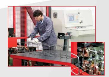
The lateral positioning of the stirrups on the welding heads allows a simple, fast and safe loading. The three welding heads allow the maximum freedom in positioning the electrodes, between stirrups and longitudinal wires. It is possible to use stirrups of different diameter wire, arranged automatically with fix or variable pitch.
