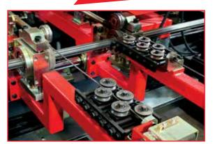
The sustaining longitudinal wires are straightened and driven by groups of independent rollers, guaranteeing a continuous cycle and eliminating downtime between a cage and the other.
