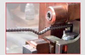
The "V" shape of the longitudinal wires (patented system) allow to keep them inside the stirrup structure. The obtained pre-cage therefore complies with the designed standards and is much more rigid, then the following handling will not deform the structure.
