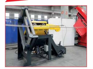
Pre-straightening and feeding unit equipped with winch and pre-straight with motorised roller, it eases and speeds up the alignment and the insertion of the wires, particularly suitable for the large diameters.
