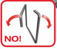
The twisting of the wire during the pulling phase create open stirrups.
