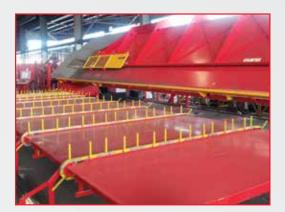
The automatic collection devices are used to maintain high levels of productivity, reducing downtime normally required for the evacuation of the products finished. Each unit can be equipped with single or multiple collection cart configuration.
