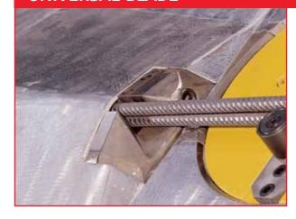
• The cutting unit utilities universal knives for all diameters processed with 4 cutting faces.
