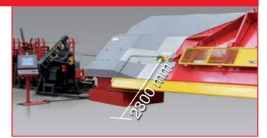
**PLANET 20 Plus** allows to get coplanar shapes and stirrups continuously closed, eliminating the dangerous manual operator intervention during the bending phase.
