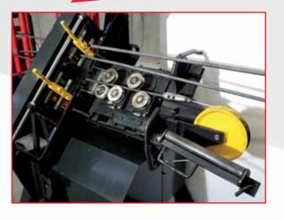
Pre-straightening and feeding unit equipped with winch and pre-straight with motorised roller, it eases and speeds up the alignment and the insertion of the wires, particularly suitable for the large diameters.
