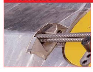
• The cutting unit utilities universal knives for all diameters processed with 4 cutting faces.
