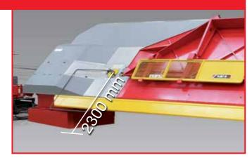
PLANET 16 Plus allows to get coplanar shapes and stirrups continuously closed, eliminating the dangerous manual operator intervention during the bending phase.
