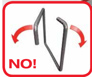
The twisting of the wire during the pulling phase creates shapes not co-planar and open stirrups.
