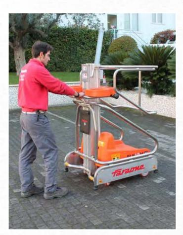
The manual traction platform Elevah 40B allow you to work up to 4 m in safety.
