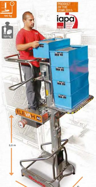
The **self propelled** machine for safe picking activities to up to 4 metres, with **automatic elevation** and a 24 volt battery.
