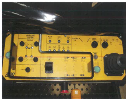
Quadro comandi in piattaforma On-platform control panel
