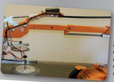
In addition to the electrical extension, the carrying arm is fitted with a manual extension arm to provide extra long reach.
