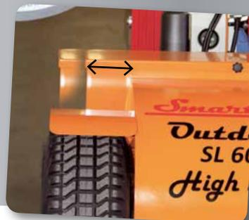
*The lift has 100 mm sideshift for accurate adjustment when fitting the window*
