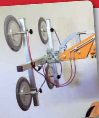
The vacuum system is separated into two vacuum circuits for highest security. Showing vacuum circuits with blue and red vacuum hoses
