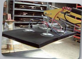
The SL 380 Midi is fitted for window and glass installation as standard, but can be supplied with a special device for lifting, e.g. heavy fire doors and gates.
